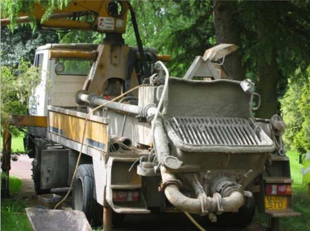
Special vehicle pumps concrete around to fill in the foundations.
